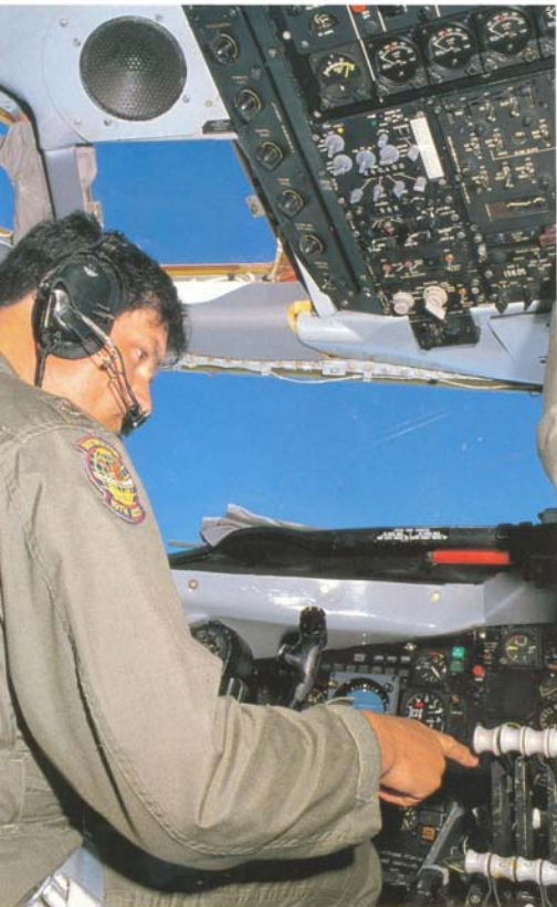
Aircraft captain Major Mike Lauro and copilot Major Bruce Monk take EC-135H callsign AXE 10 up into the blue at 28,000 feet and 270 knots after taking off from Mildenhall with 120,000 pounds of gas aboard (note complex fuel system schematic, switchgear and tank contents gauges above power levers to left of Monk's knee). The EC-135H's four Pratt & Whitney TF33-PW102 (JT3D) turbofans burn about 12,000 pounds of fuel per hour
